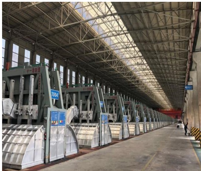
Figure 12. NEUI600 potline in Inner Mongolia aluminium smelter.
