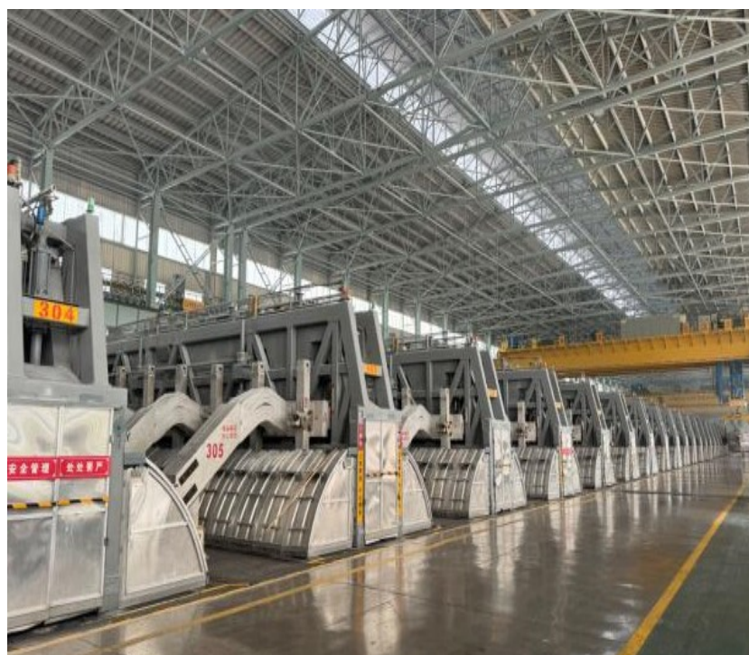
Figure 9. A NEUI600 potline in Shandong Weiqiao Aluminium & Power Co., Ltd. aluminium smelter.
