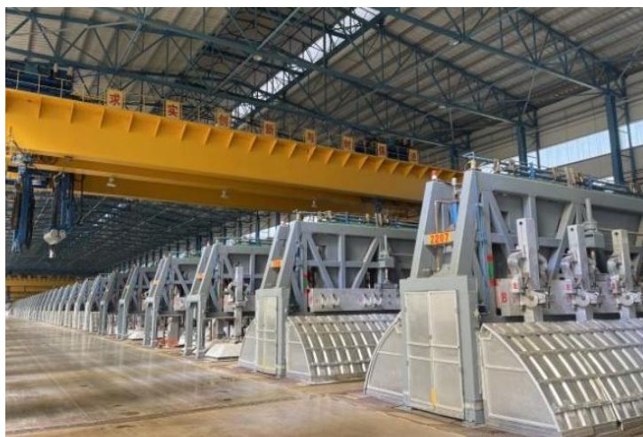
Figure 10. NEUI600 potlines in Yunnan Hongtai aluminium smelter.
